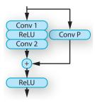
Fig. 7. Residual blocks. We employ residual blocks in the G-buffer encoder and RAD modules. The blocks consist of convolutional layers (kernel size 3) with spectral normalization [92] and ReLUs. Changes in channel width or downscaling are performed in  $\mathtt{Conv}\ 1$  and  $\mathtt{Conv}\ P$ . If channel width and resolution are constant, the projection via  $\mathtt{Conv}\ P$  is omitted.
