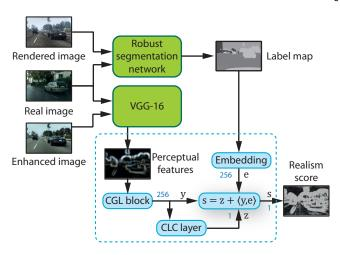
Fig. 9. Perceptual discriminator. Realism of enhanced images is evaluated via a perceptual discriminator. It consists of pretrained robust segmentation (MSeg [72]) and perceptual (VGG [93]) networks. These provide high-level semantic information via label maps and perceptual feature tensors. The maps and tensors are ingested by discriminator networks, which produce a realism score map. For clarity, we only show a single discriminator network, indicated by the dashed rectangle.
