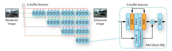
Fig. 4. Image enhancement network. We replace the batch normalization layers within HRNet by rendering-aware denormalization (RAD), forming RAD blocks (RB). Each branch of the HRNet receives a G-buffer feature tensor at a matching scale (different scales are coded by color). Original feature streams are shown in gray. We omit initial stem convolutions as well as transition and fusion layers for clarity.
