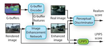
Fig. 3. Our approach is built around an image enhancement network that transforms a rendered image. In addition to the image, the network ingests G-buffer feature tensors at multiple scales. The tensors represent rendering information from a conventional graphics pipeline, encoded by a G-buffer encoder network. Both networks are trained jointly via an LPIPS loss (to retain the structure of the rendered image) and a perceptual discriminator (to maximize the realism of the enhanced image).
